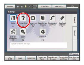
**Step 14.** Confirm the version of the software. The Version must be the same version number or higher than the version noted in Step 11 of Receiving the Project Data from the (Damaged) COBOTTA.
