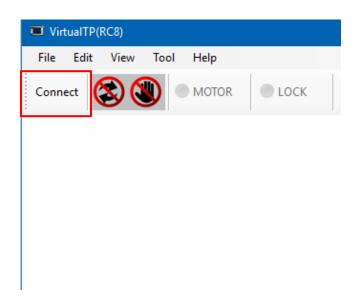
**Step 5.** Enter the IP address of the COBOTTA and then choose [Connect].
