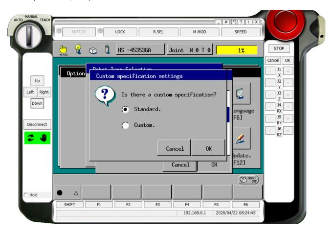
**Step 10-** This concludes the Teach Pendant setup and on this screen the high lighted red area should reflect the same as the robot type on the base of the robot. Turn controller power of at this time for the following three steps.
