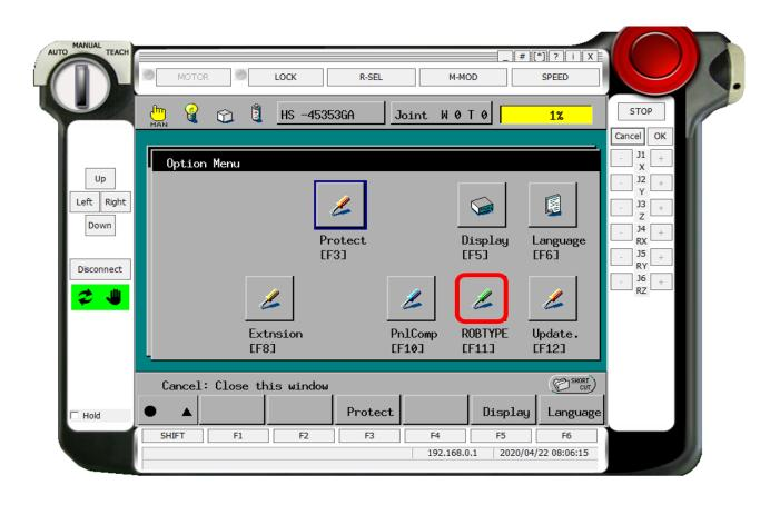
**Step 4**- When you select ROBTYPE an input keypad will appear and you will need to enter: **1967103** then press the "OK" button on the input pad.
