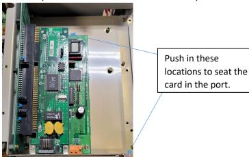
5. When gold contacts are no longer visible, the card is seated, install port cover screw removed in step 2 to secure the card.
