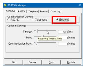
8. Select the Ethernet tab and populate the IP address of the controller. You made note of this address in step 8 of controller configuration. Select "Update" after you have this information populated. The telephone icon should now have a red "E" next to the phone to designate the controller and WCII are now connected.
