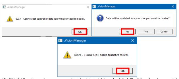
13. Click "ok" on the .systemmanager noting the data batch transfer failed. The failure is only present due to the failure to receive vision data. The rest of the project will have been received in the project.
